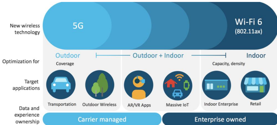
Figure 4 – Complementary role of 5G and WiFi 6 interworking facilitated by OpenRoaming. Source: Cisco, 2020
